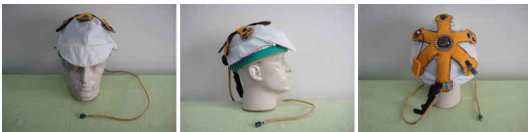
Figure 10 – Details of aCap: three different views of the wearable, with a switch plugged on one of the four plugs on the back of the device.
