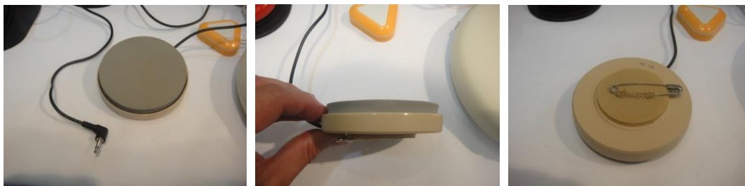
Figure 5 – A switch that can be used by a tetraplegic user. It is activated by head and shoulder movements: it has a soft sponge in front of it and a pin on its back that can be used to fix it to user clothes.
