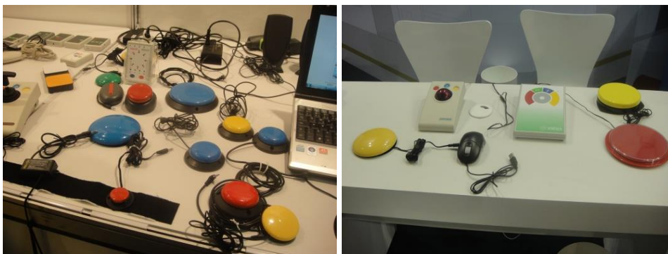
Figure 2 – AT retailer booths at a national accessibility product fair. Most of the buttons above (left picture) are single on-off switches to be plugged in other AT devices, like adapted mice or joysticks (right picture).
