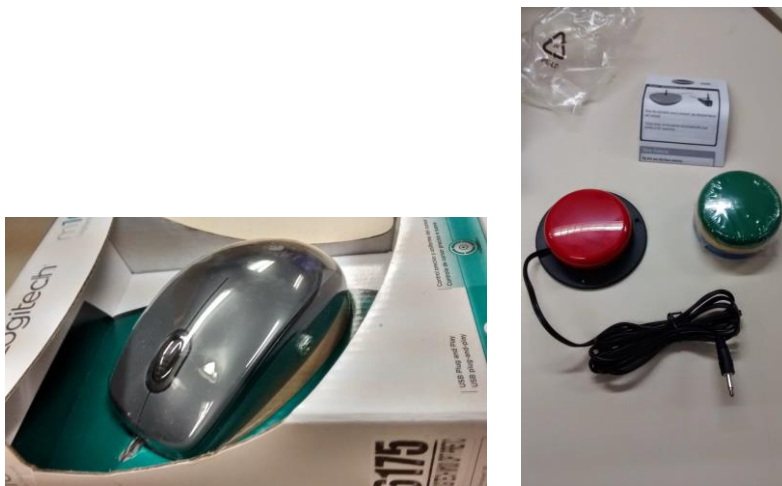
Figure 4 – An adapted mouse (left) and an accessible switch (right) to be plugged in it. The mouse and the switch use a standard P2 plug, which allows the switch to be exchanged by different models, which can better suit users' different preferences, kinds and degrees of disabilities (see Figure 5 below).
